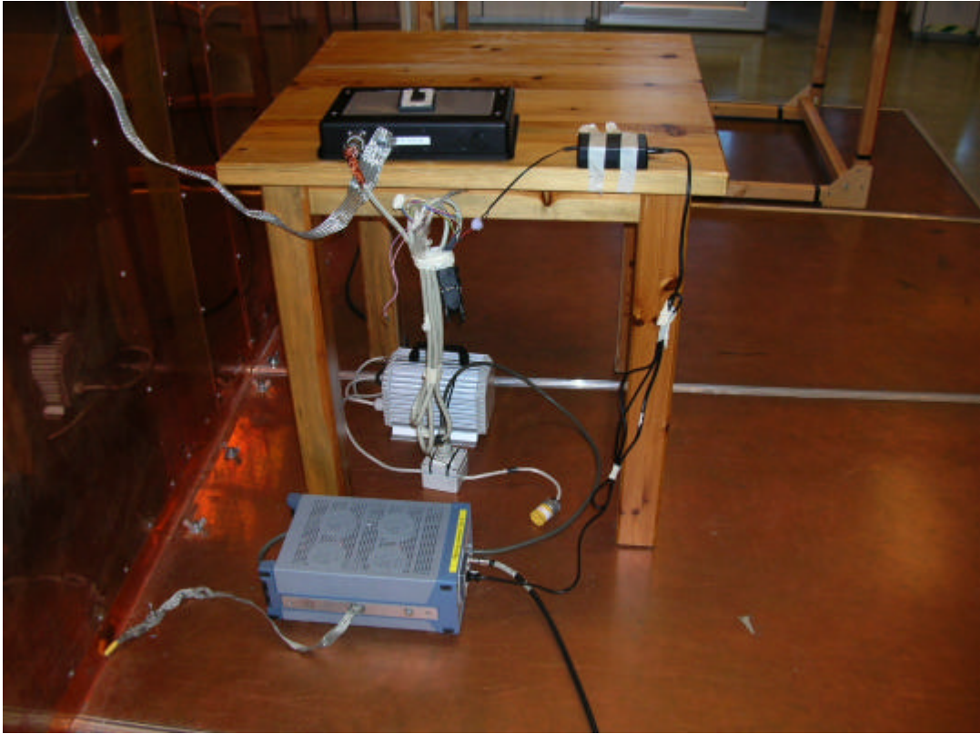
S1566 – Conducted disturbance voltage at AC terminal
