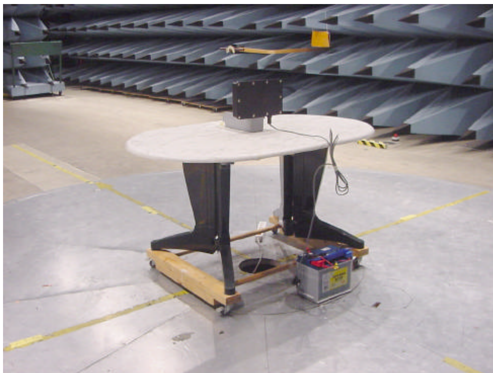
Semi-anechoic shielded chamber (30 – 1000 MHz), type S1566
