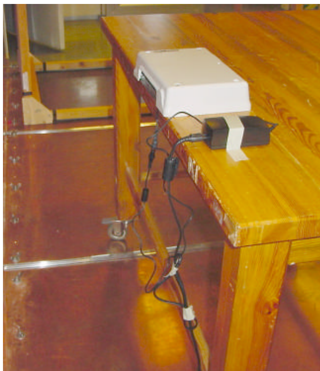
Conducted disturbance voltage 0,150-30 MHz, type S1500
