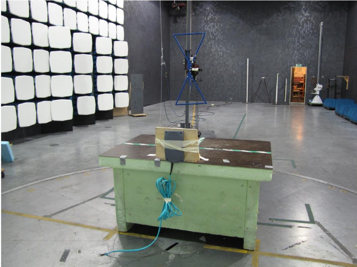
Test set up radiated emission 30 MHz – 1GHz
