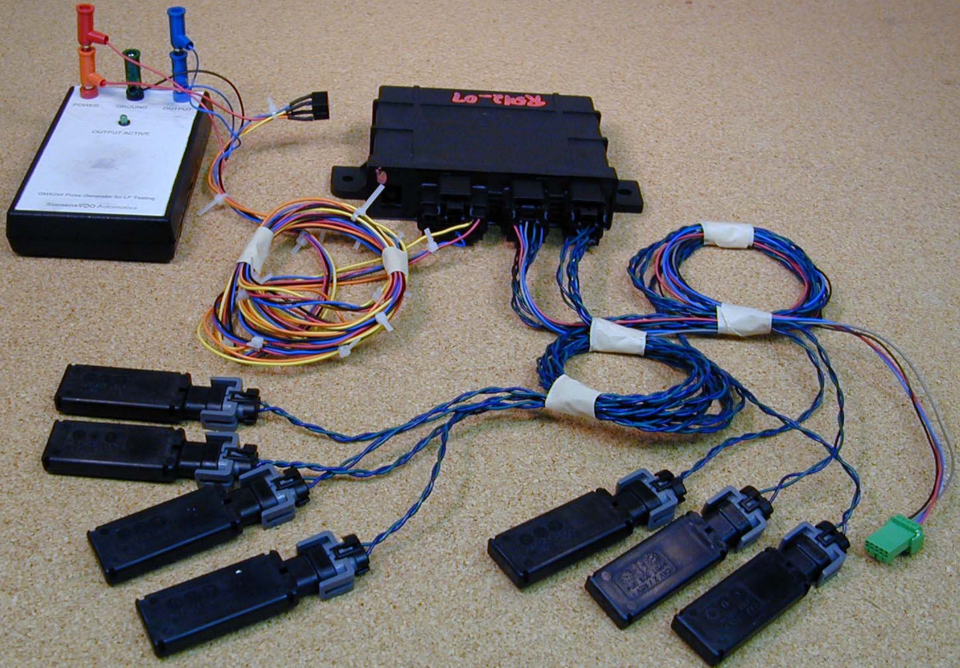
DUT with harness, test box, and activator coils
