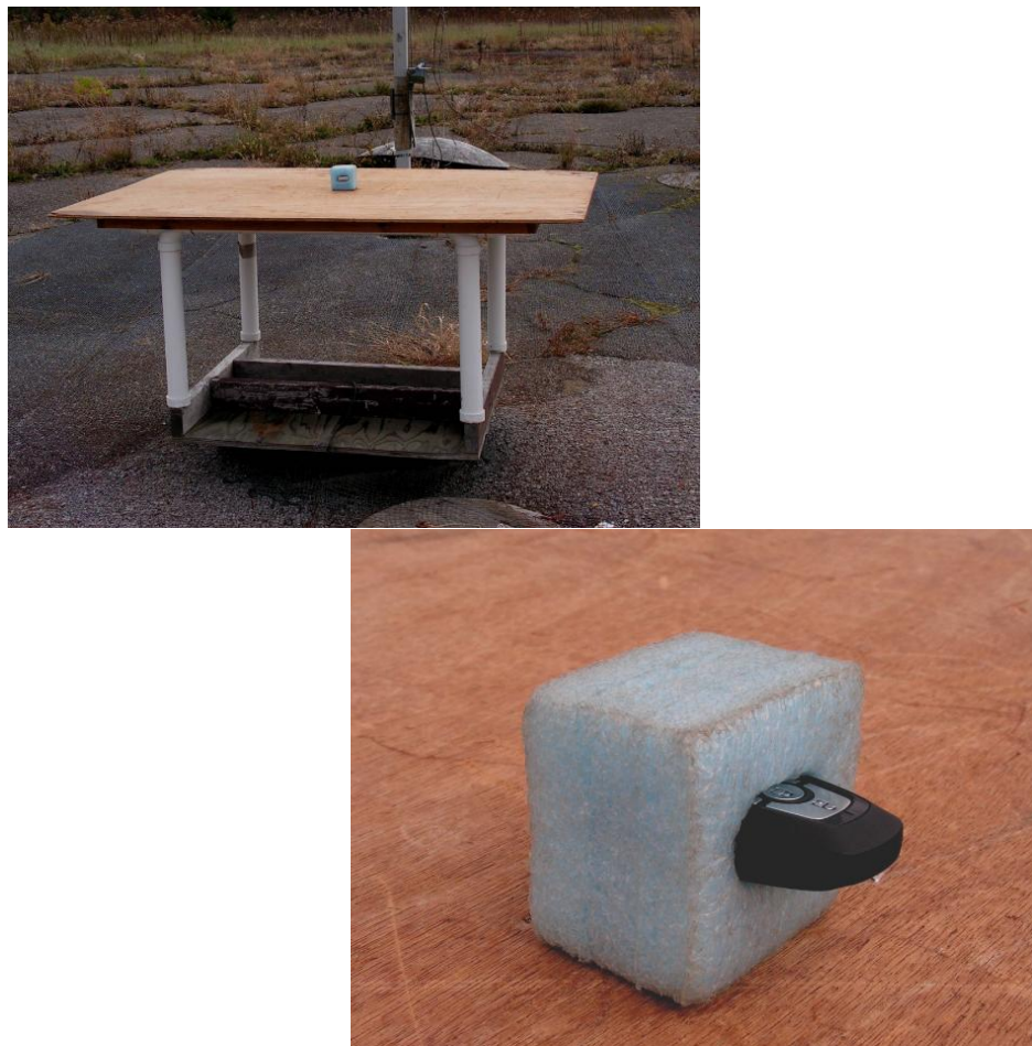
Figure 4: Radiated Emissions Test Setup Photograph(s).
