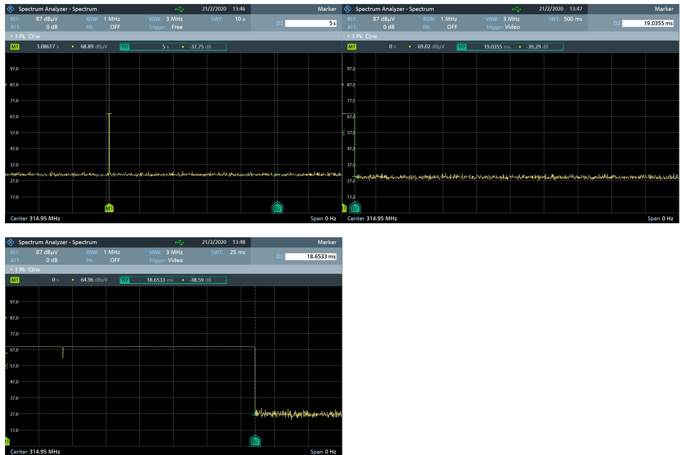
Figure 5: Fundamental Emission Pulsed Operation.
