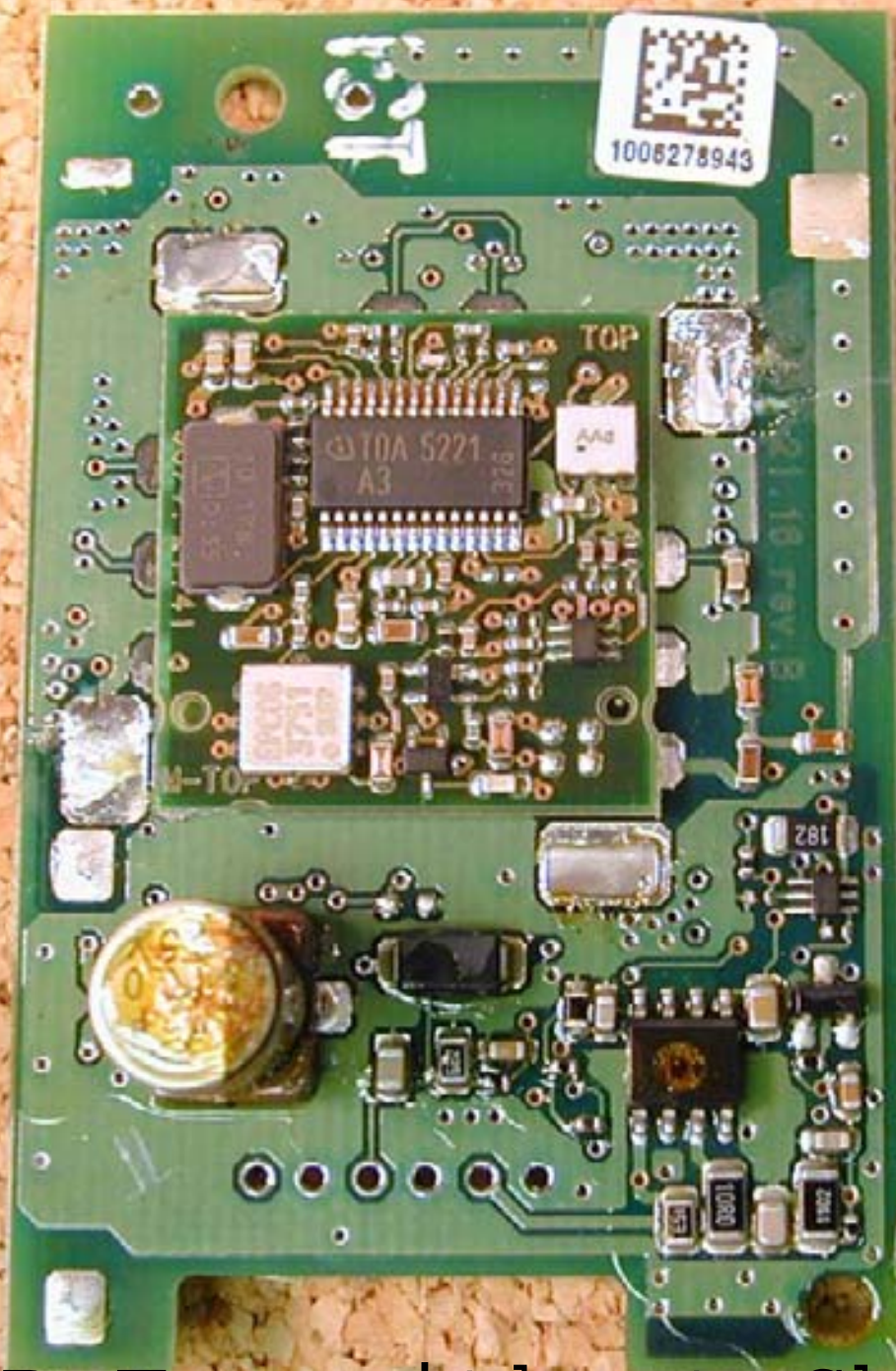
RS PCB Top without Shielding
