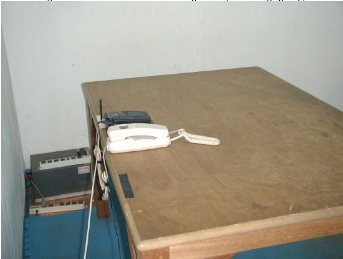
Fig. 2 Conducted Emissions Test Configuration (Base Charging only)
