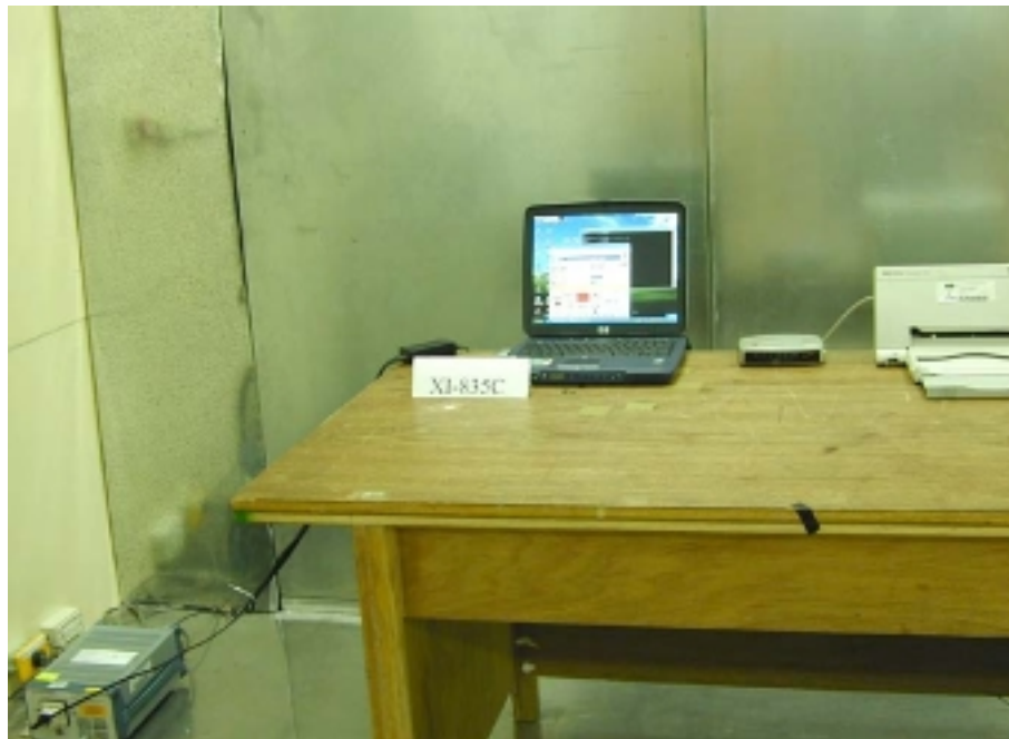
Photo 1: Conducted Test Set-up (front)
