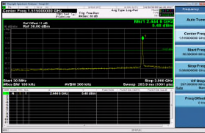
802.11g: Spurious Emission Test Data CH-Mid
