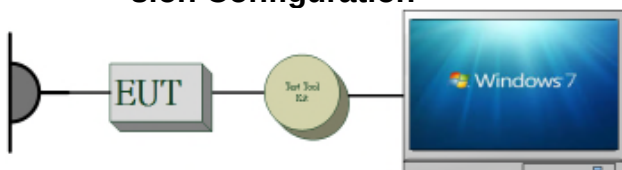
Fig. 2-2 Conducted (Antenna Port) Emission Configuration
