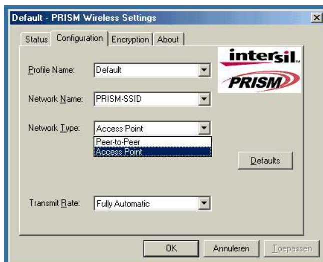
fig, 03: WLAN network type setting window
