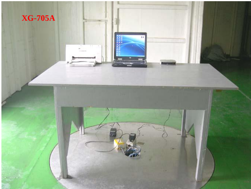
Photo 2: Radiated Emission Test Set-up
