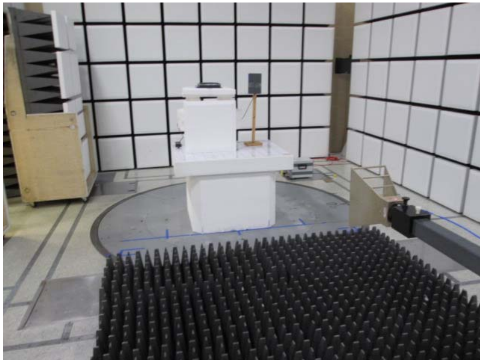
Test Set Up Photo –A1001 Antenna (above 1GHz)
