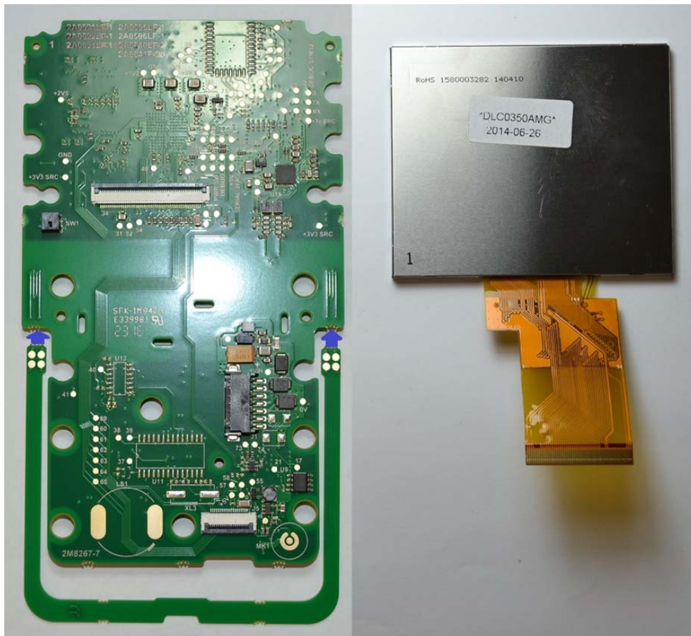
T21 Mifare - PCB (rear side) and LCD
