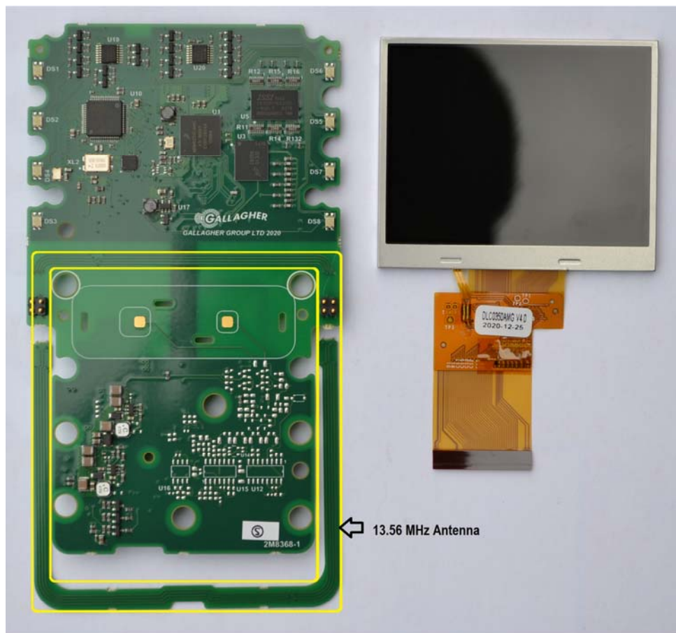
T21 PIV Reader - 13.56 MHz Antenna. PCB (front side) and LCD
