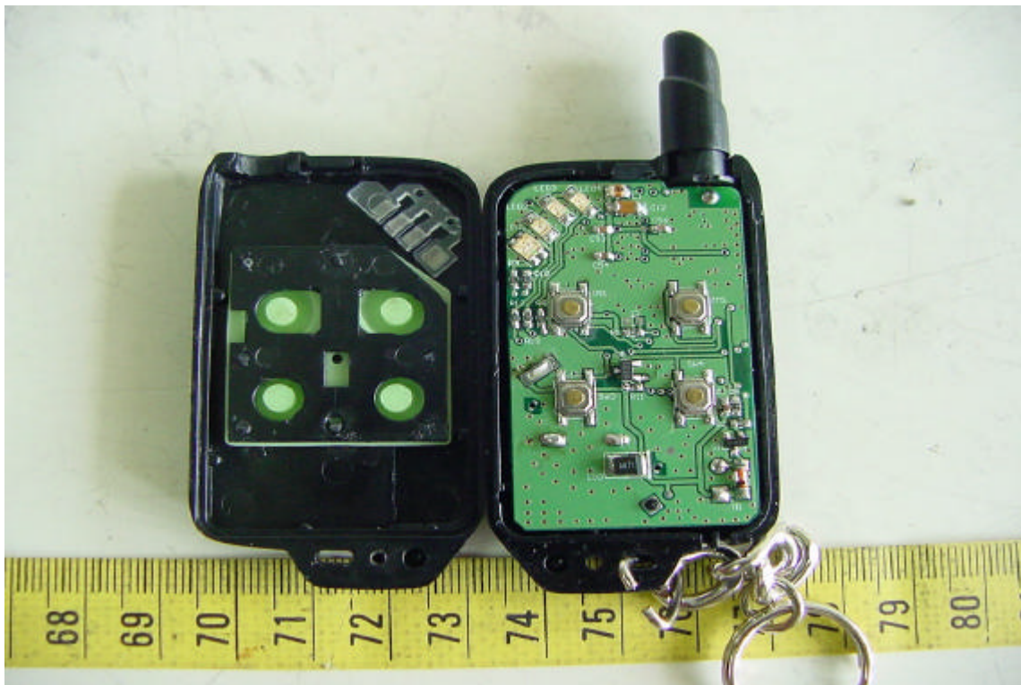
Internal View of EUT
