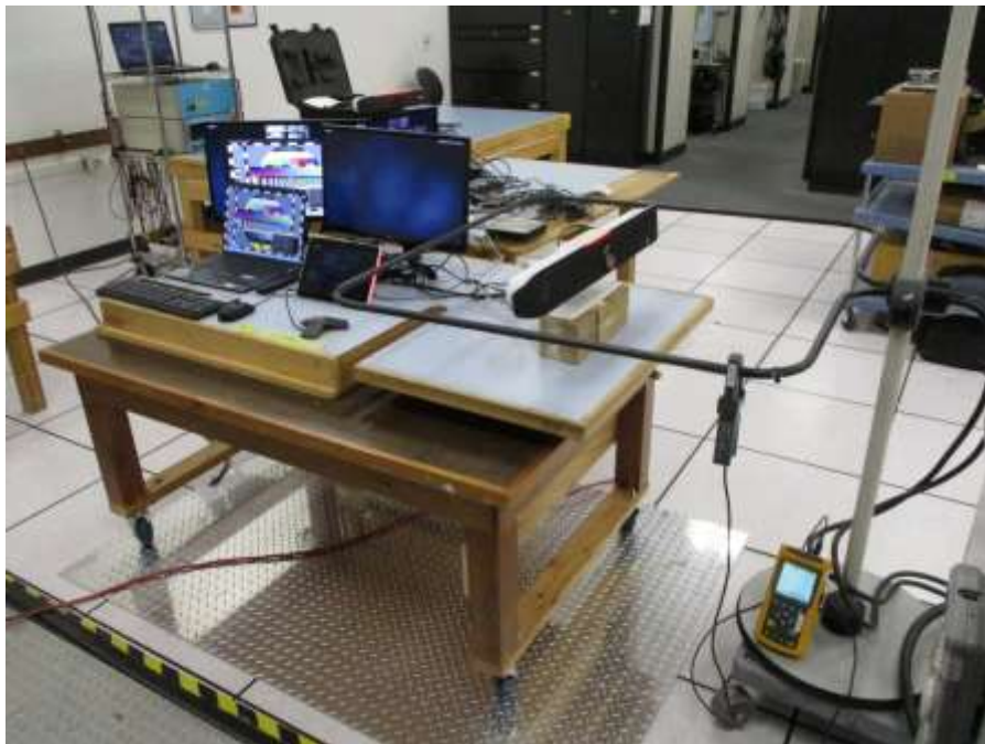
Photograph 45. Power Frequency, Magnetic Field, X-Axis Orientation Test
