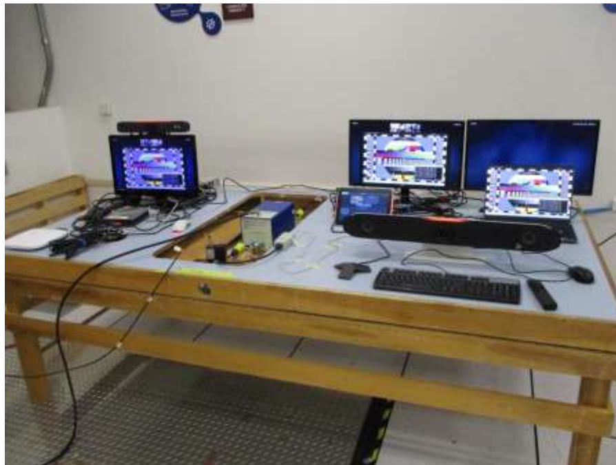
Photograph 39. Conducted Immunity, AC Mains Overall Test Setup
