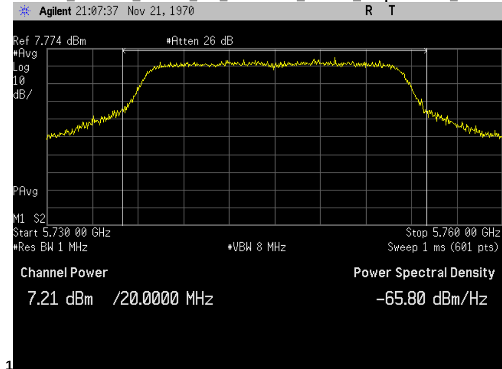
U-NII-3_5745MHz_Low Ch_149_20MHz BW_a-mode_Output Power_Port
