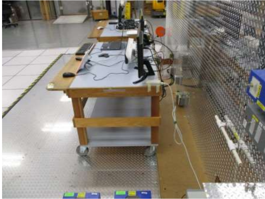
Photograph 3. Conducted Emissions, AC Mains, Side View
