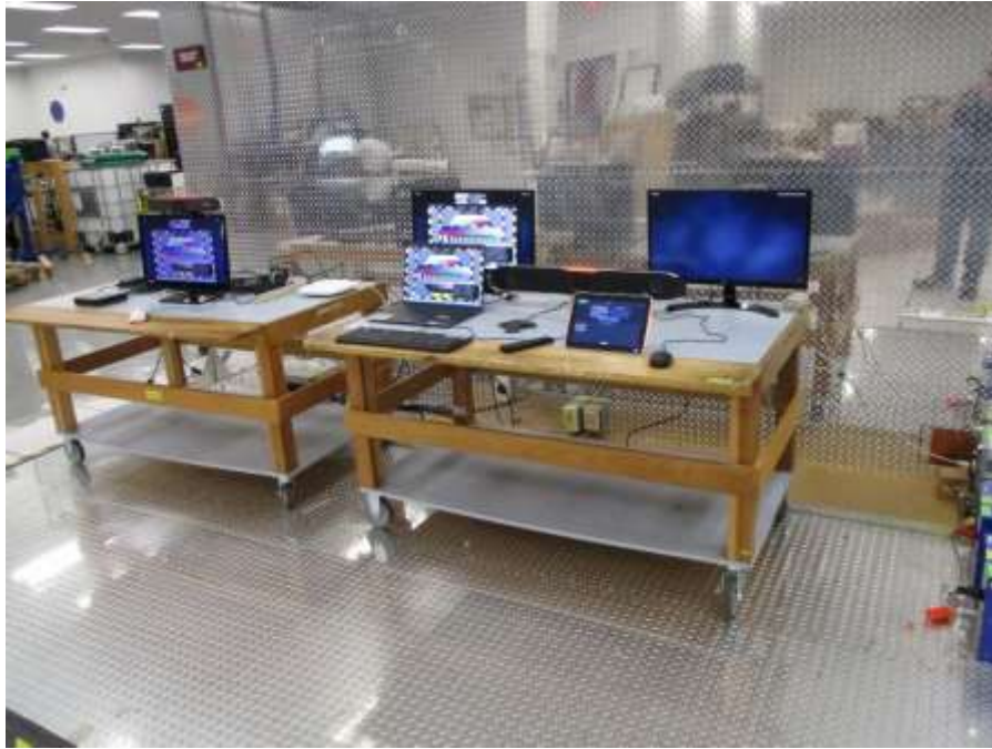
Photograph 1. Conducted Emissions, AC Mains, Front View
