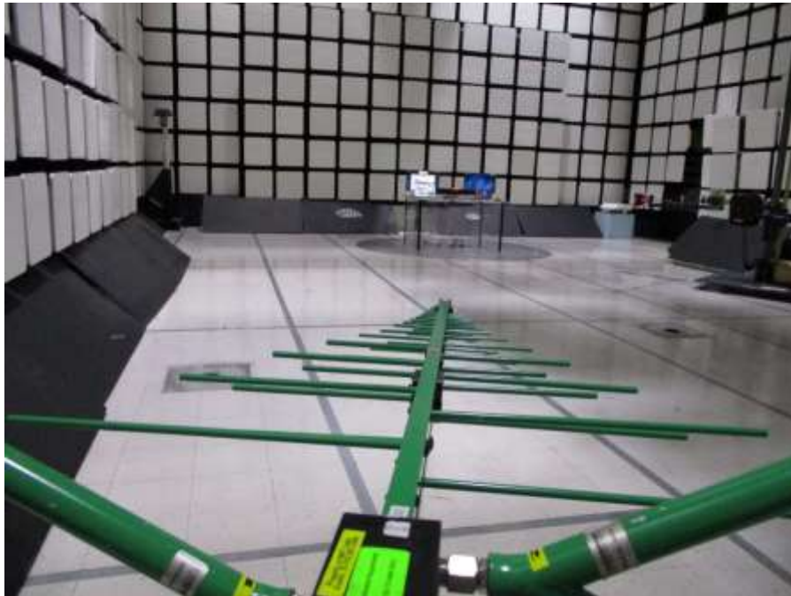
Photograph 6. Radiated Emissions, 30 MHz – 1000 MHz, Antenna View
