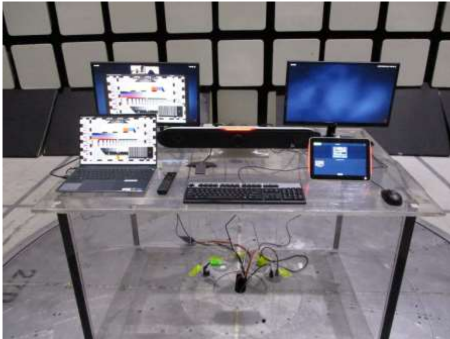
Photograph 4. Radiated Emissions, 30 MHz – 1000 MHz, Front View
