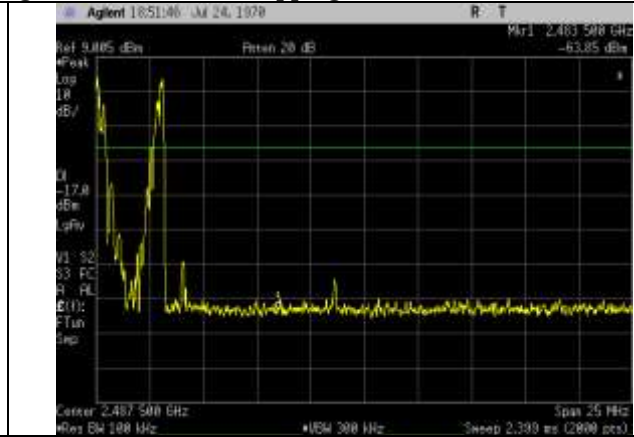
2480MHz, Upper Band Edge, GFSK
