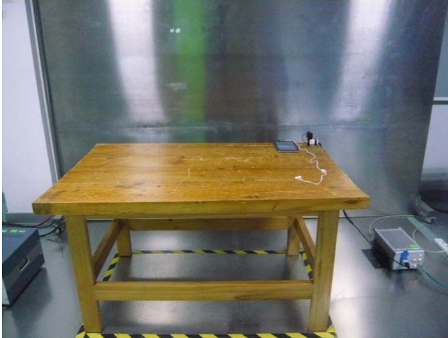
Conducted Emissions – Front View (Charging&Playing)
