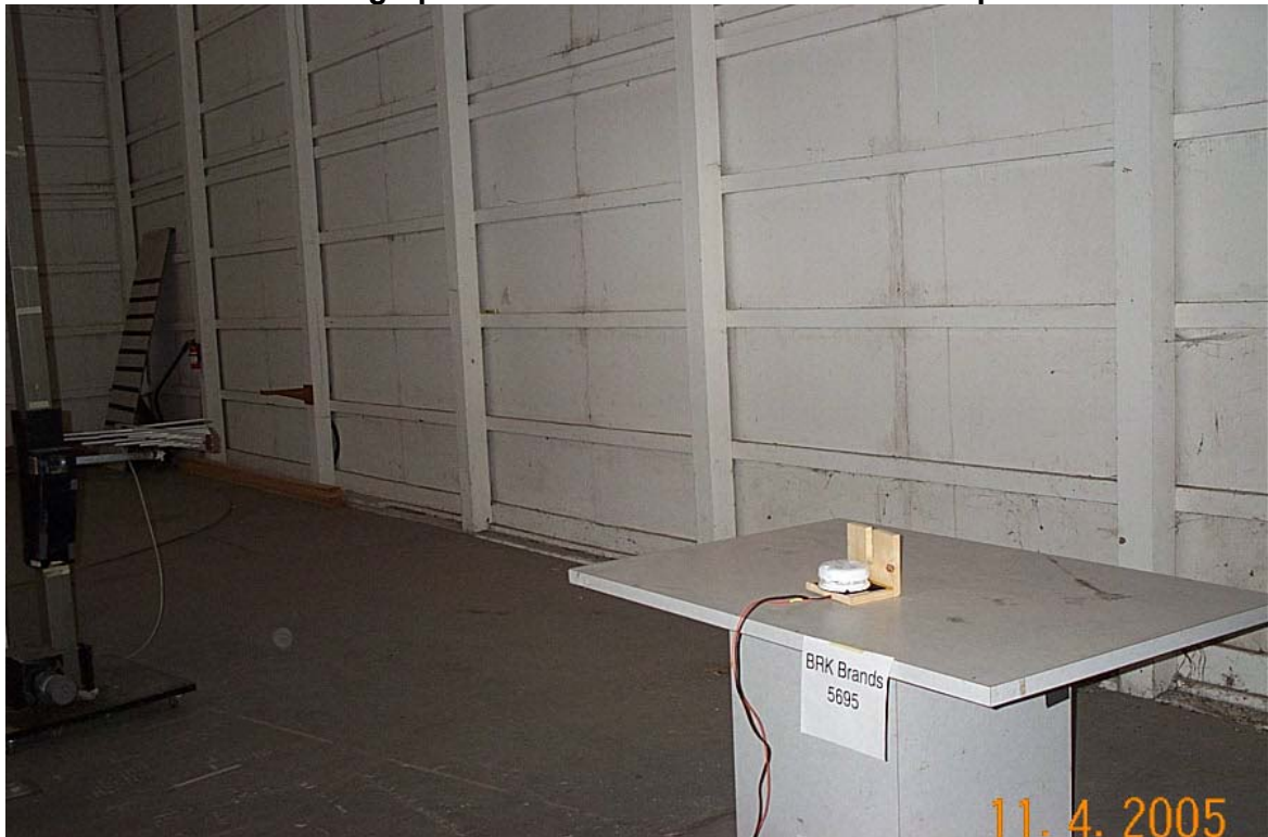
Photographs of Radiated Emissions Test Setup
