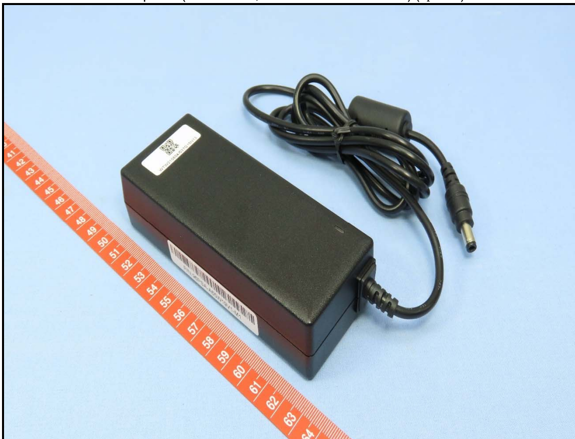
Adapter 2 (Brand: FSP, Model: FSP065-DBCM1) (option)
