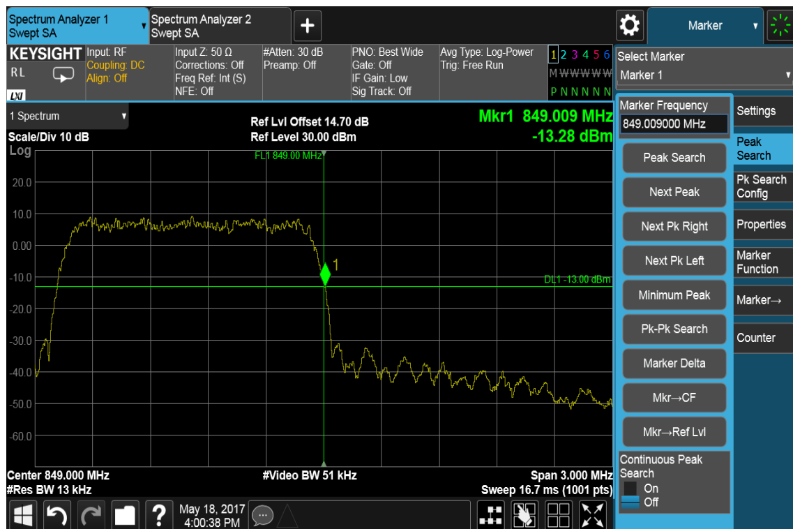
Figure 10-2: Band Edge emissions –CDMA / BC0 / CH 777
