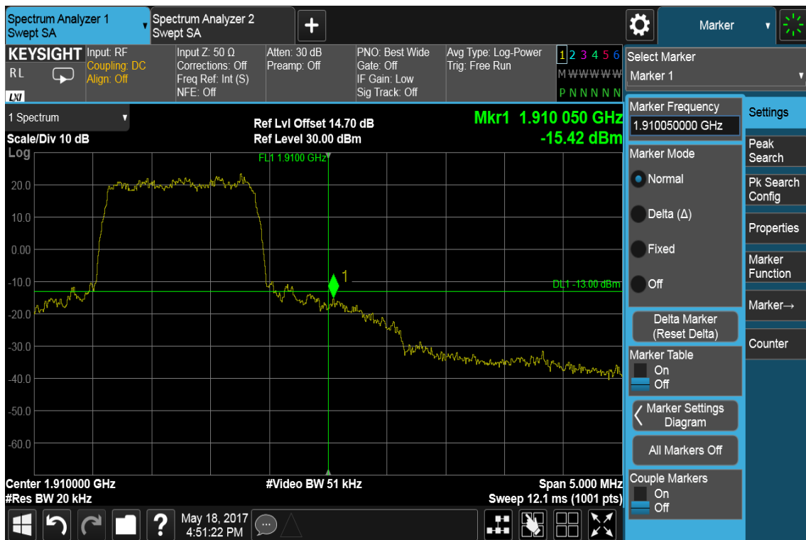
Figure 11-2: Band Edge emissions –CDMA / BC1 / CH 1175
