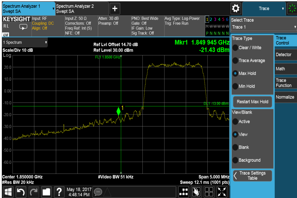
Figure 11-1: Band Edge emissions –CDMA / BC1 / CH 25
