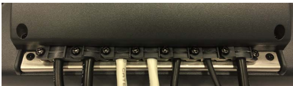
Fig. 6.9: Cable cover closed and screwed together
