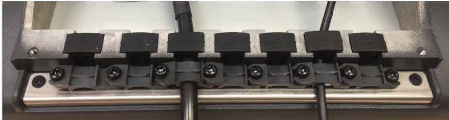
Fig. 6.1: Rubber seal inserted in the cable compartment
