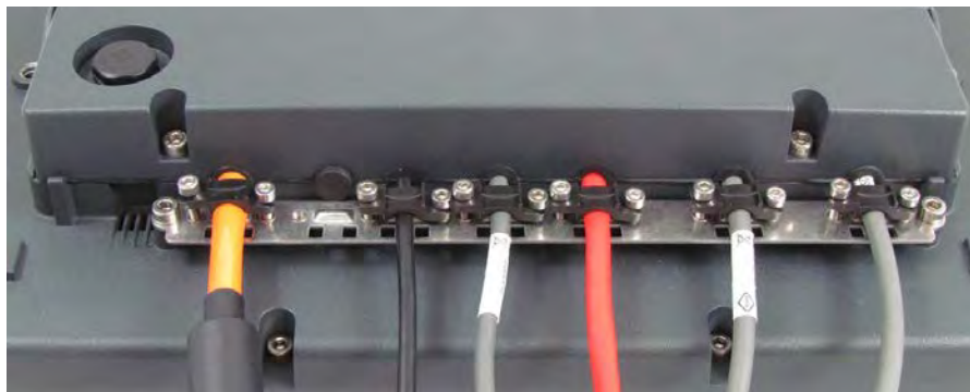
Fig. 12.9: Cable cover closed and screwed together
