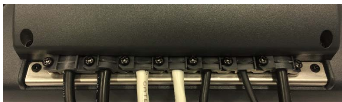
Fig. 6.9: Cable cover closed and screwed together
