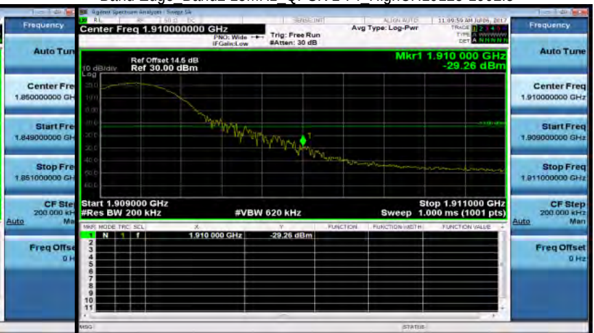
Band Edge Band2 15MHz QPSK 1 74 HighCH19125-1902.5
