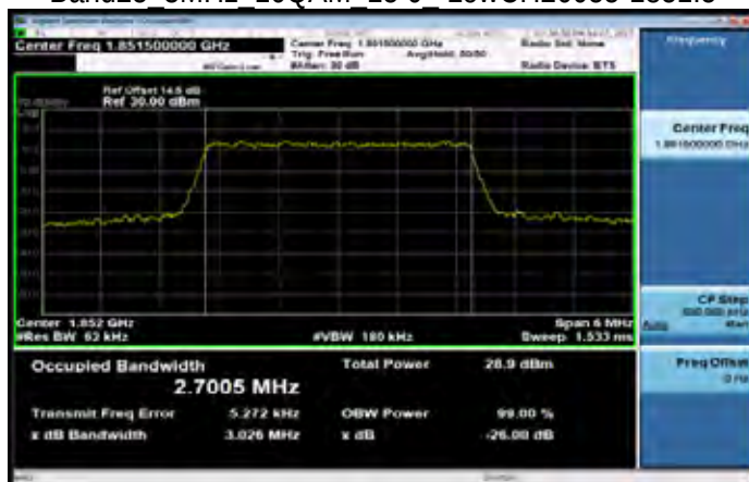
Band25 3MHz 16QAM 15 0 LowCH26055-1851.5
