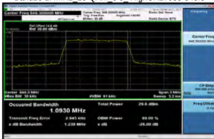
Band26 1.4MHz 16-QAM 6 0 HighCH27033-848.3
