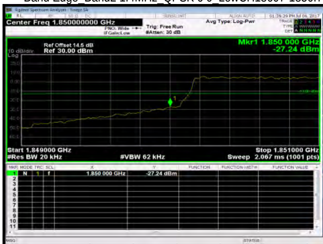
Band Edge Band2 1.4MHz QPSK 6 0 LowCH18607-1850.7
