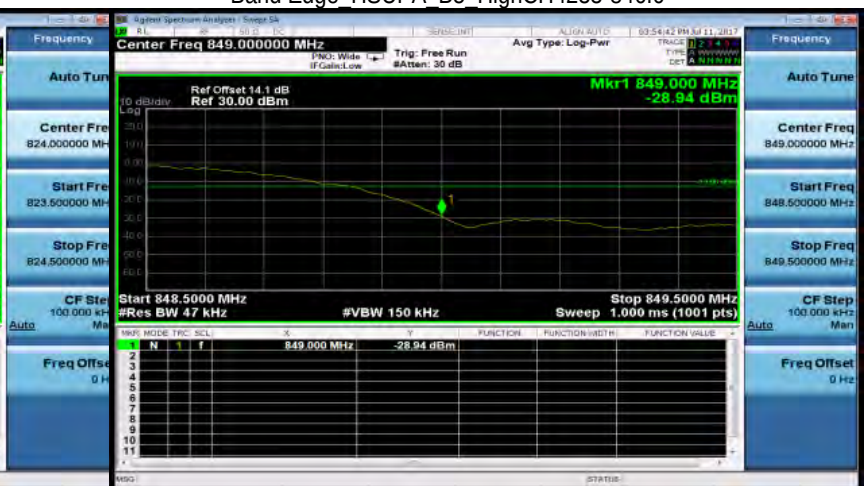
Band Edge HSUPA B5 HighCH4233-846.6
