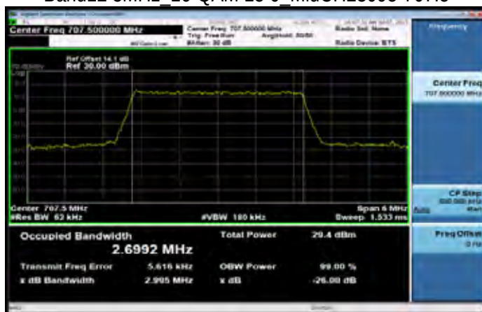
Band12 3MHz 16-QAM 15 0 MidCH23095-707.5
