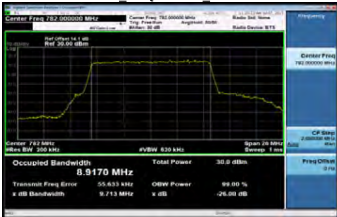
Band13 10MHz 16-QAM 50 0 MidCH23230-782
