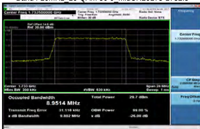
Band4 10MHz 16-QAM 50 0 MidCH20175-1732.5
