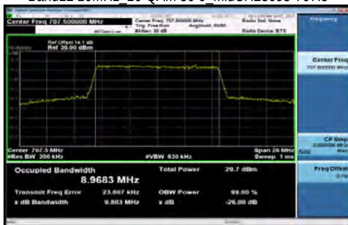
Band12 10MHz 16-QAM 50 0 MidCH23095-707.5
