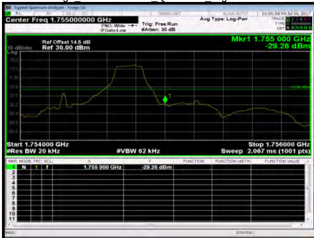
Band Edge Band4 1.4MHz QPSK 1 5 HighCH20393-1754.3
