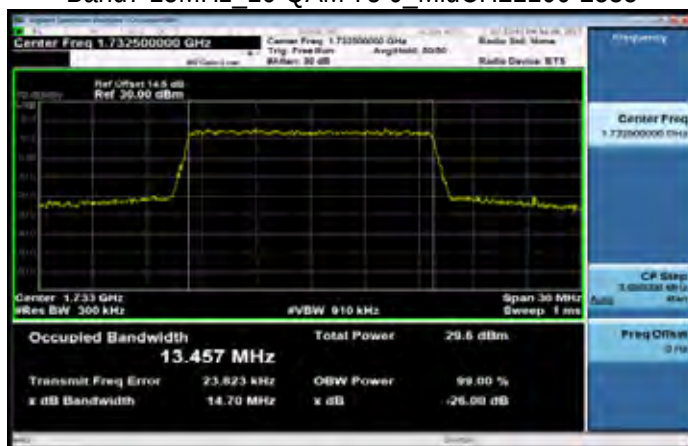
Band7 15MHz_16-QAM 75 0_MidCH21100-2535
