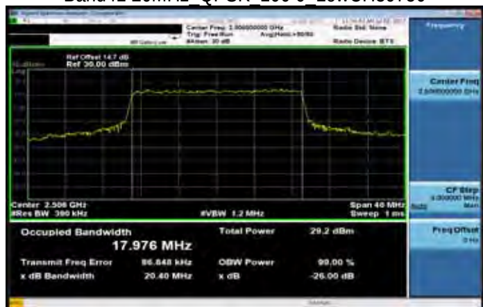
Band41 20MHz QPSK 100 0 LowCH39750
