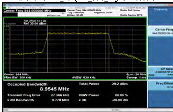
Band26 10MHz 16-QAM 50 0 HighCH26990-844
