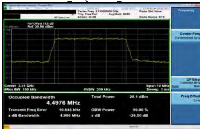
Band30 5MHz_16-QAM 25 0_MidCH27710-2310
