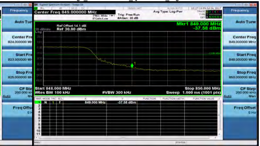
Band Edge Band5 10MHz QPSK 50 0 HighCH20600-844
