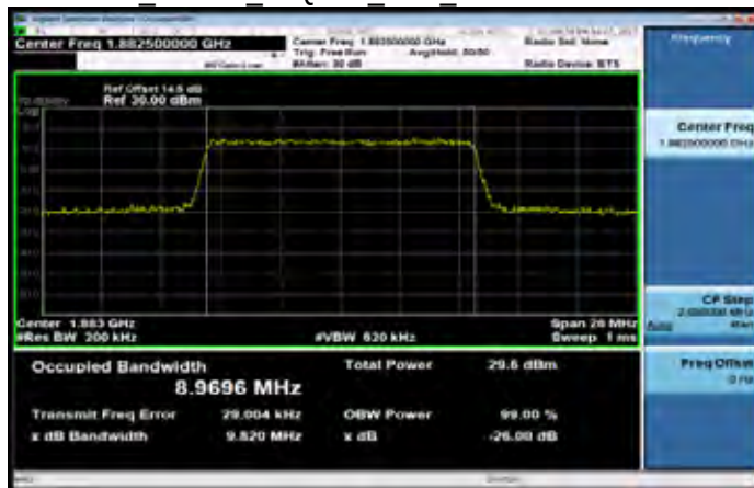
Band25 10MHz 16QAM 50 0 MidCH26365-1882.5
