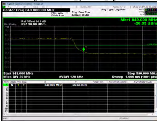
Band Edge_Band5 3MHz_QPSK 15 0_HighCH20635-847.5
