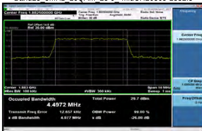
Band25 5MHz 16QAM 25 0 MidCH26365-1882.5
