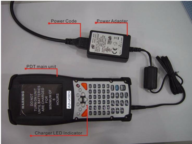
When charging the battery pack, the charge indicator on the PDT turns **Red**. After the battery pack is fully charged, the indicator turns **Green**.
