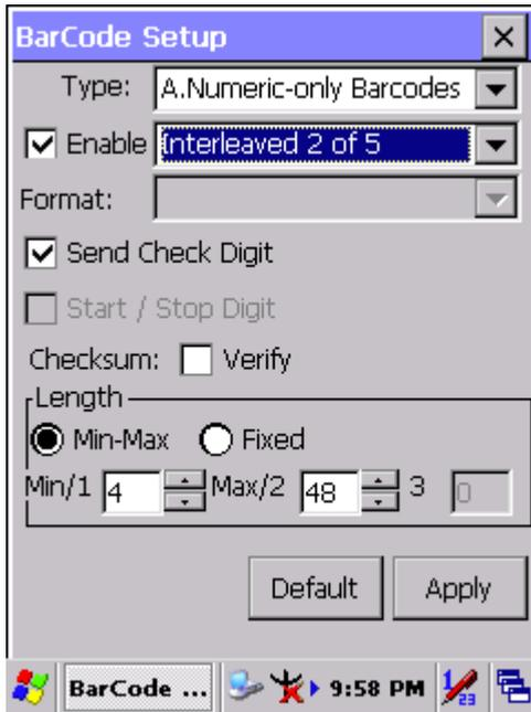
Figure 3.12: Interleaved 2 of 5
