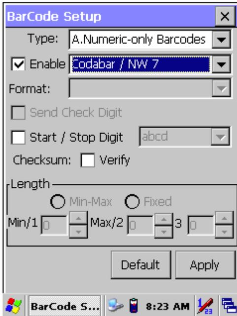
Figure 3.15: Codabar / NW7
