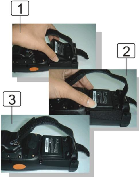
4. Replace the battery cover by inserting the top first, and then press the bottom in firmly. Turn the locking screws (right and left) upwards to secure the cover to the PDT.
