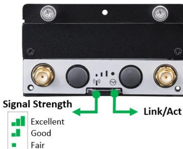
Figure 10: FIO Patch type Antenna installation
