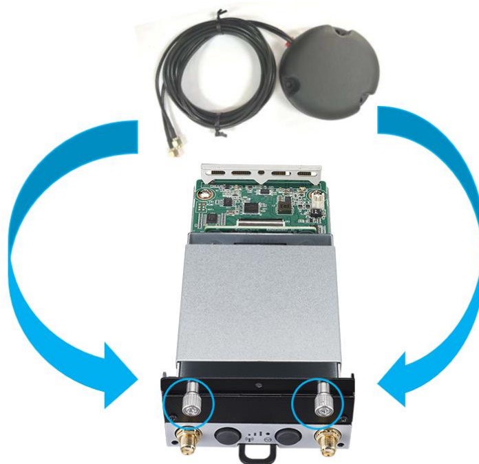
Figure 9: Patch type Antenna installation
