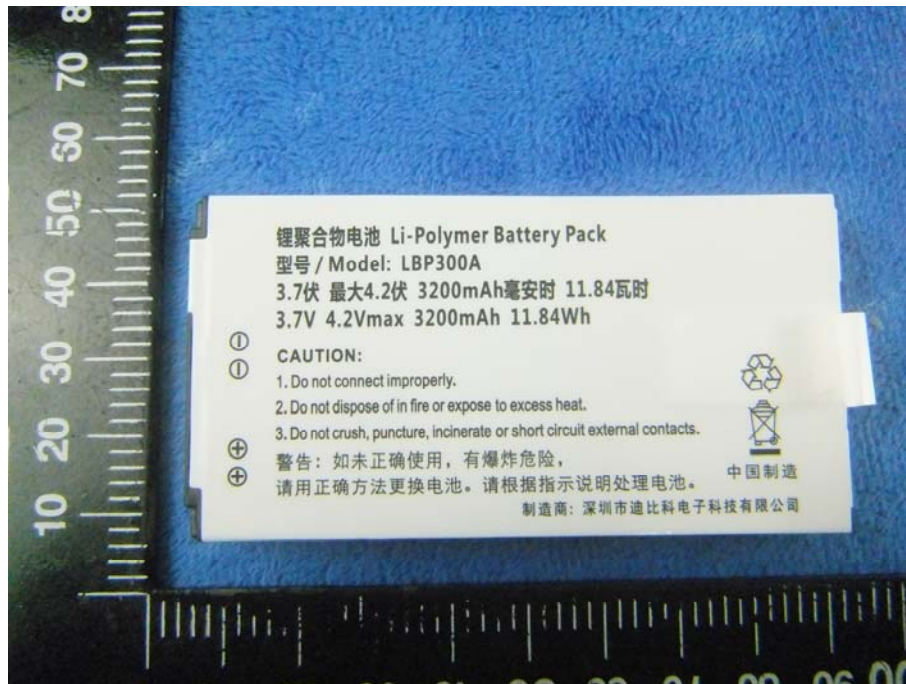
Battery - Front View
