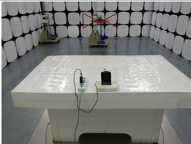
Conducted Emissions Test Setup Front View
