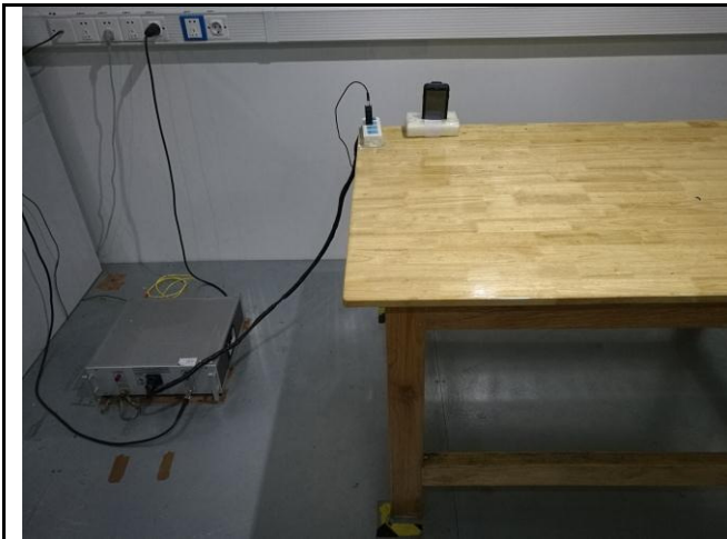
Conducted Emissions Test Setup Front View
