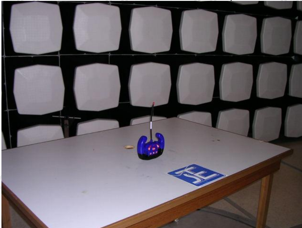
Measurement of Radiated Emission Test Set Up
