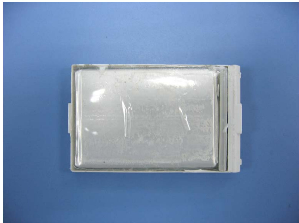
Internal view of battery
