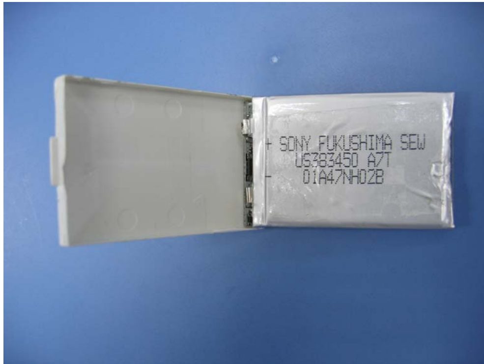
Internal view of battery
