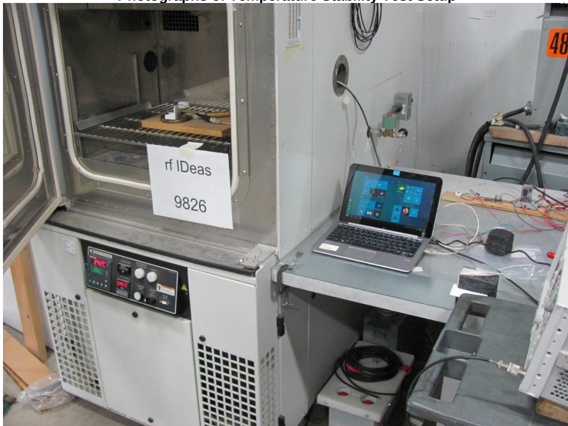
Photographs of Temperature Stability Test Setup
