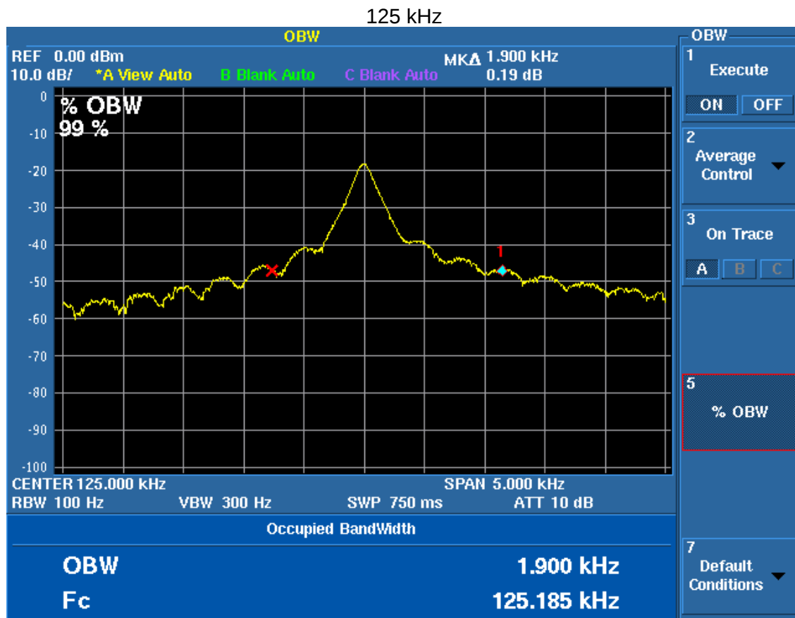
Figure 3. Occupied Bandwidth Plot
