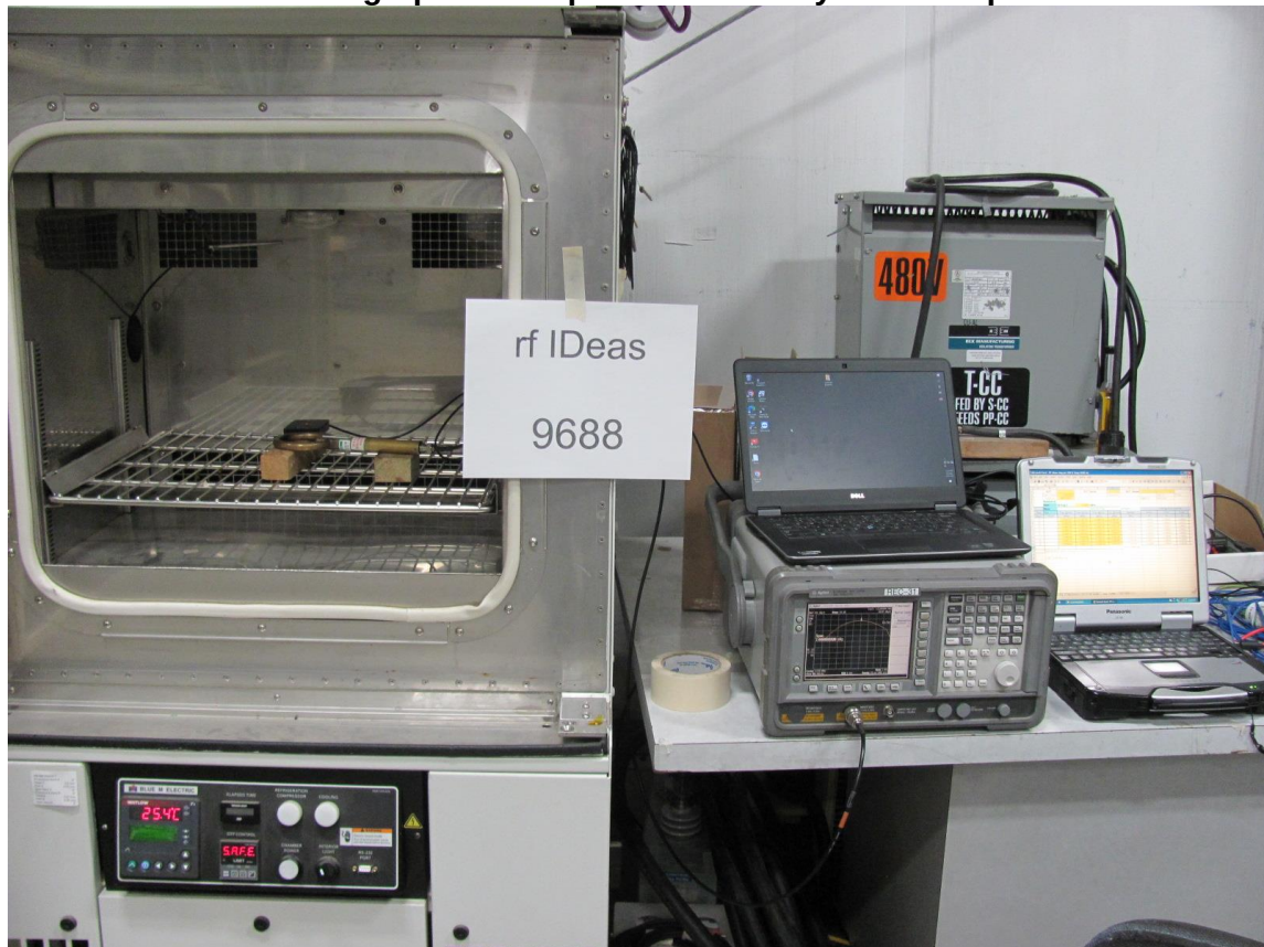
Photograph of Temperature Stability Test Setup
