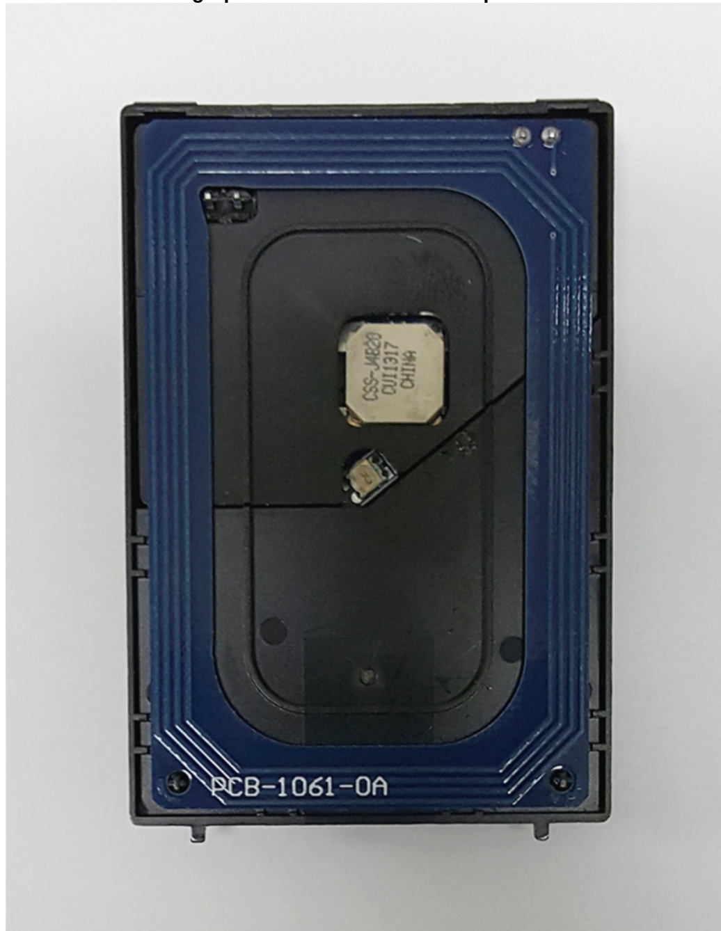
Photograph of Antenna Board: Component side
