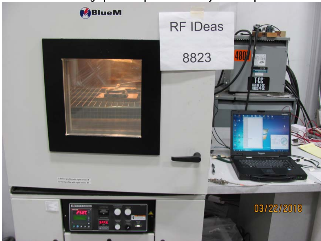
Photograph of Temperature Stability Test Setup
