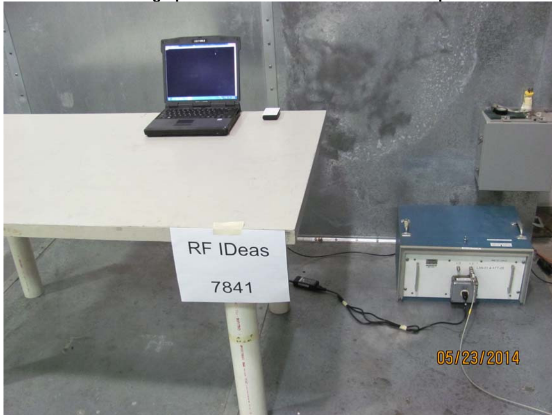
Photograph of Conducted Emissions Test Setup
