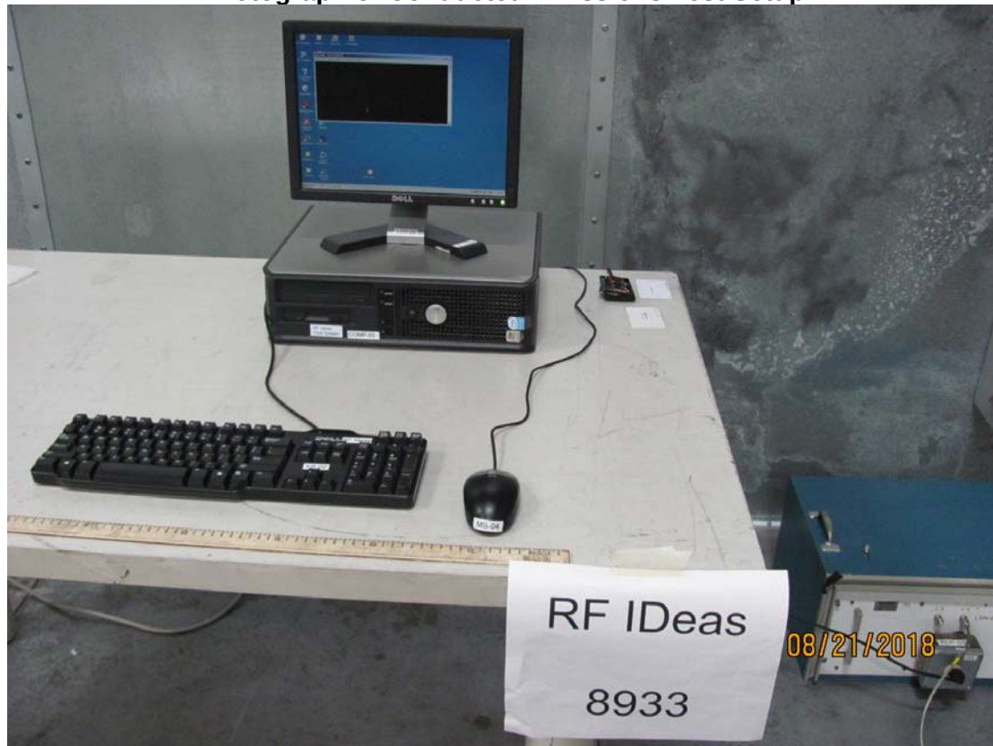
Photograph of Conducted Emissions Test Setup
