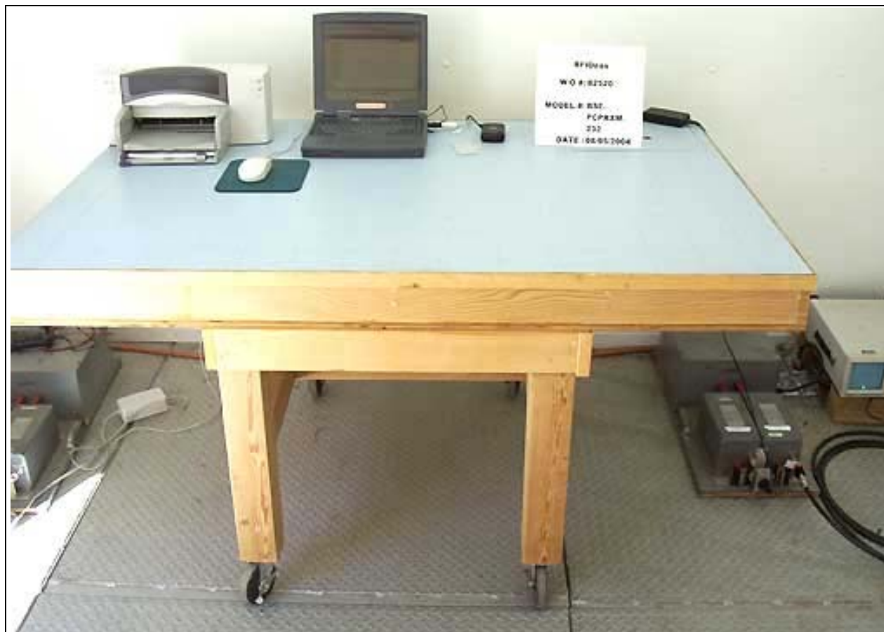
Mains Conducted Emissions - Front View - 232
