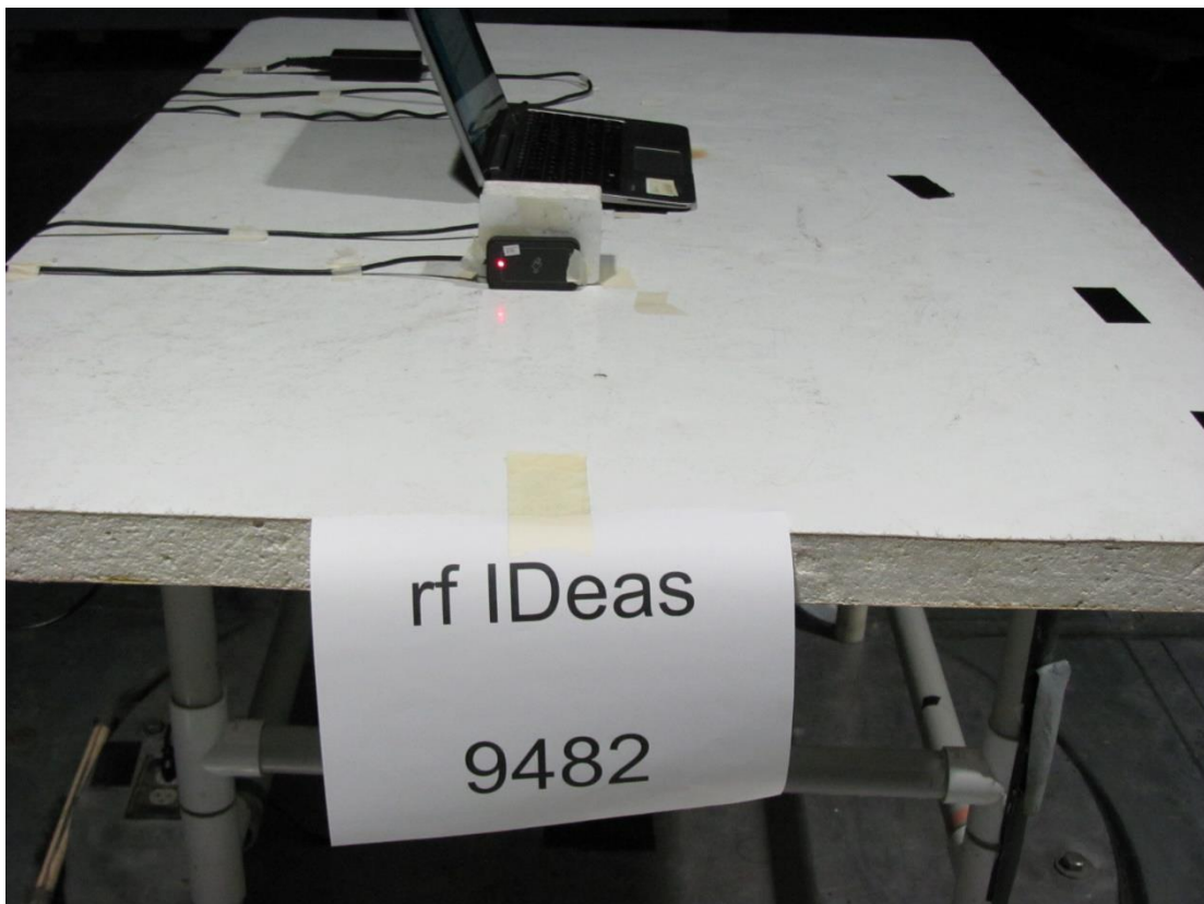
The EUT was taped to a foam block to change the orientation.
