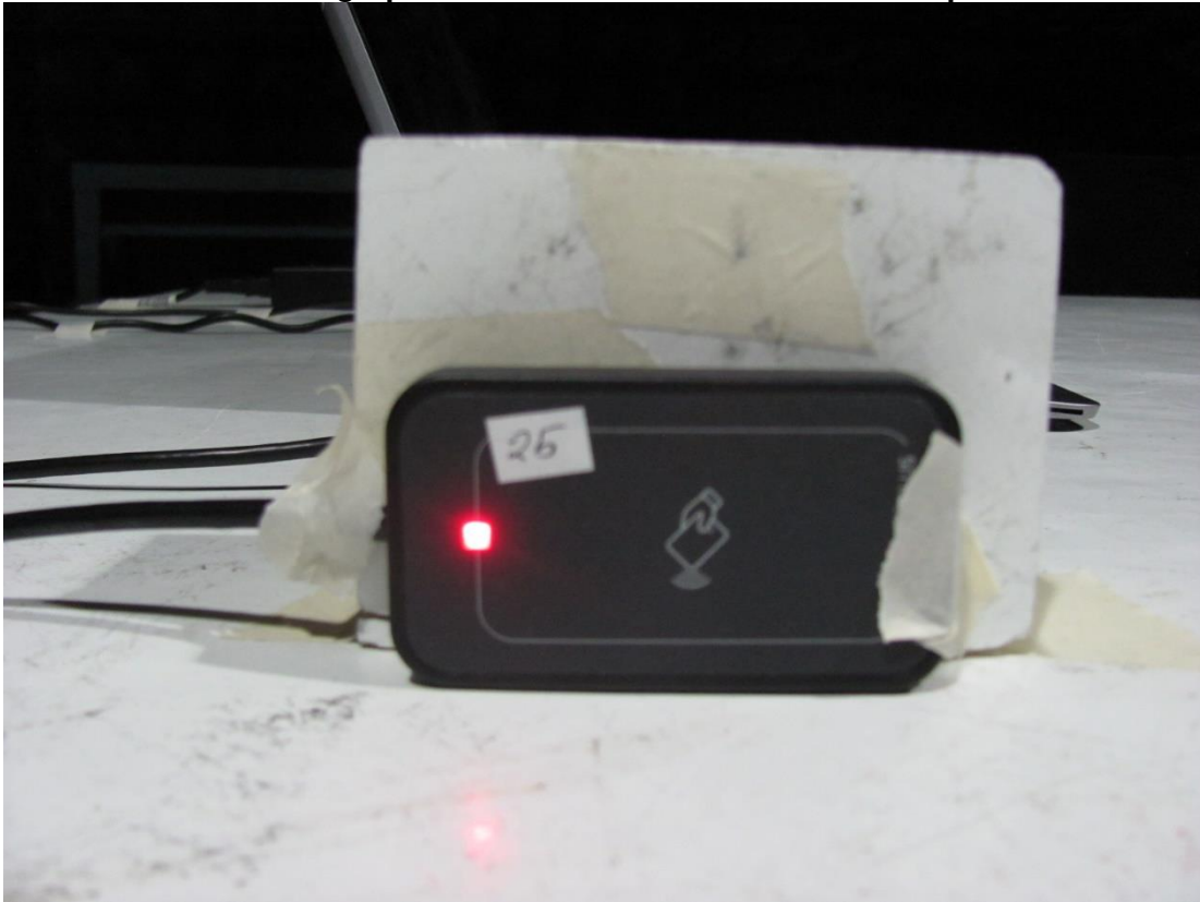
The EUT was taped to a foam block to change the orientation.
