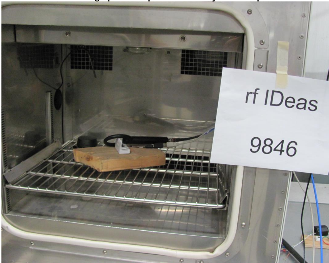
Photograph of Temperature Stability Test Setup
