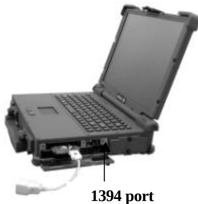
Figure 2-9 Removing IEEE 1394 Port
