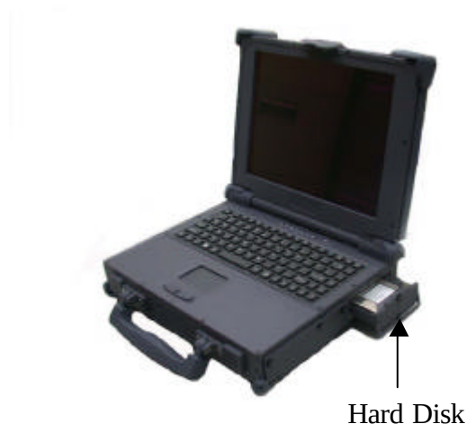
Figure 2-8 Removing a Hard Disk Drive Module
