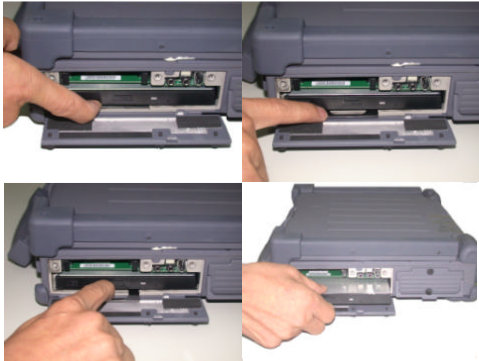
Figure 2-5 Removing a FDD/CD-ROM/DVD/COMBO /DVD RW Module
