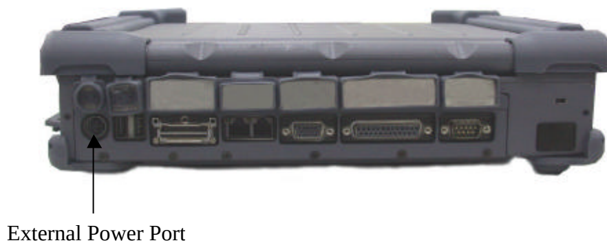
Figure 2-4 Connecting the External Power Adapter
