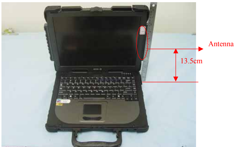
Fig. 9.3 Antenna Position for M230-4
