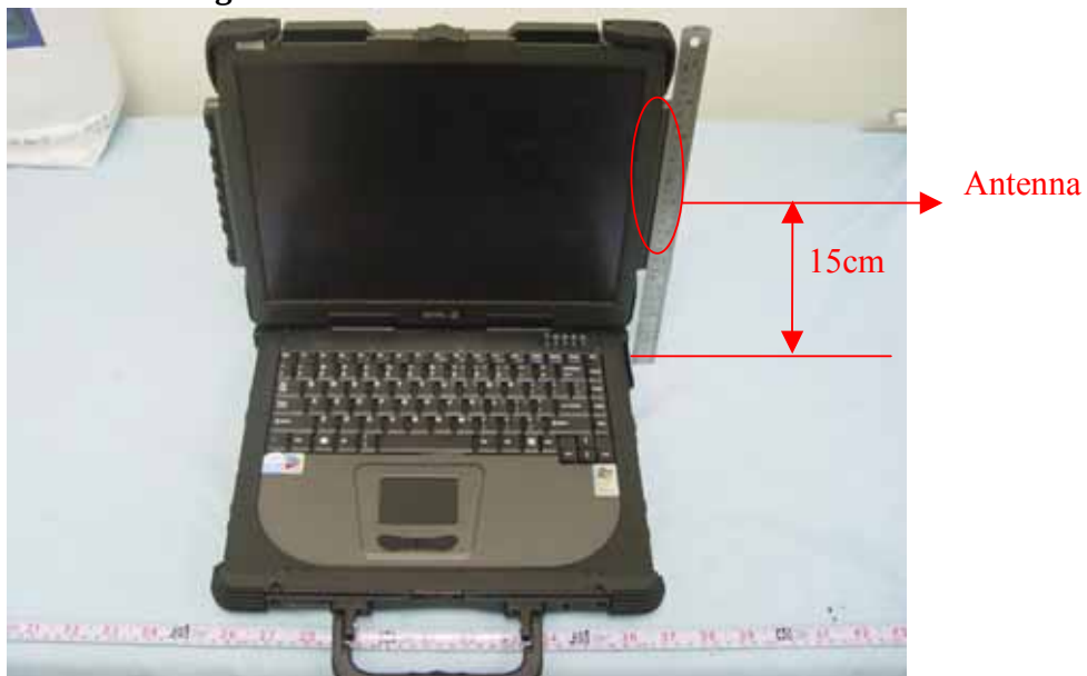
Fig. 9.4 Antenna Position for M230-5
