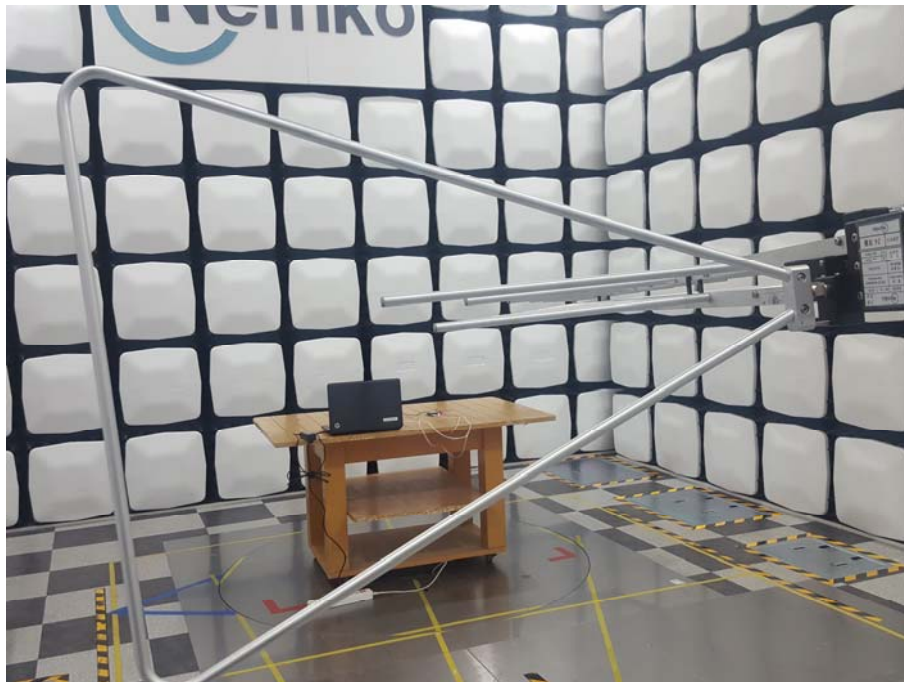
Radiated Test Picture(Rear)_Below 1GHz
