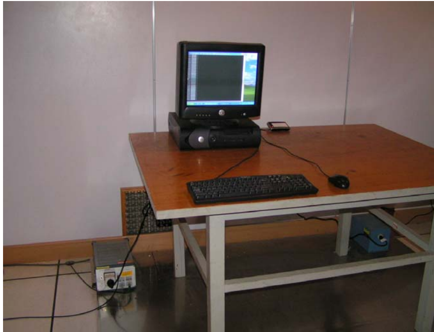
Conducted Emissions Test Set-up - Front View
