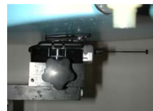
Figure 22. Body SAR Test Setup
