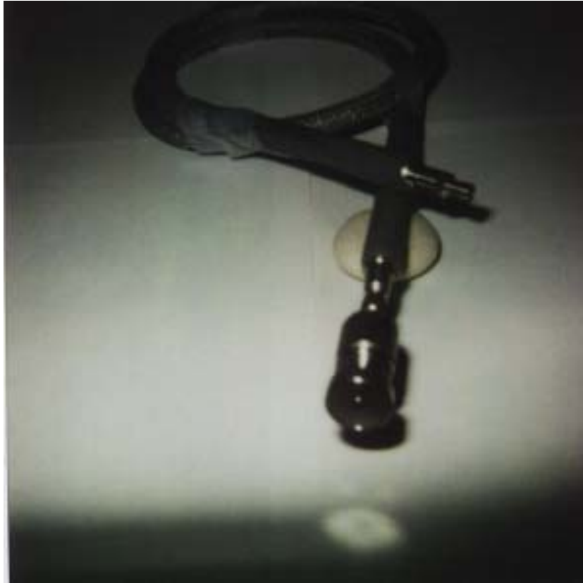
Fig. 12. Photograph of the Hewlett Packard Model 85070B Dielectric Probe. This is an open-circuited coaxial line probe.
