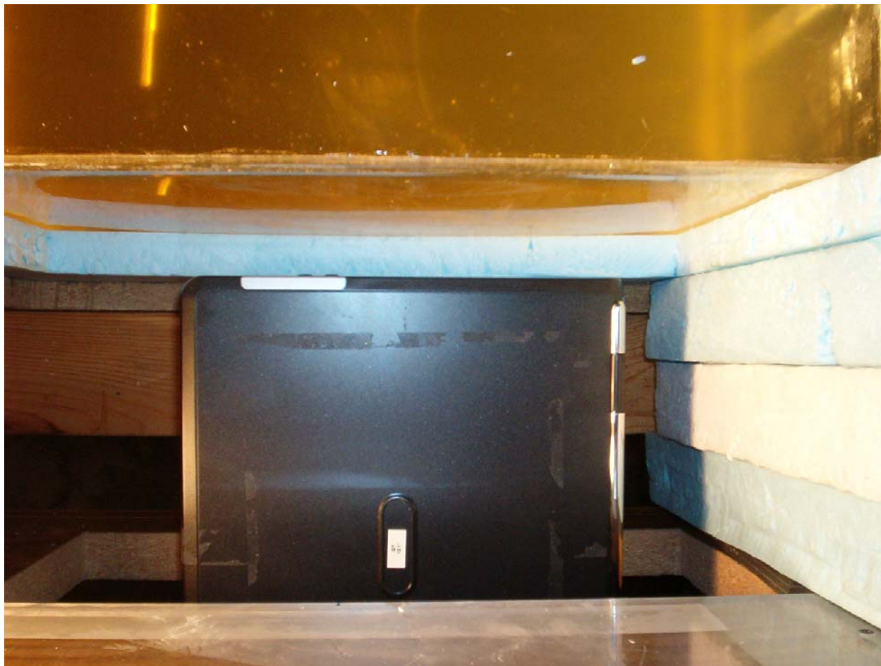
Fig. 6. Photograph of Agency Series PP2170 Laptop Computer with Ambit Microsystems 802.11a Wireless Antenna with edge of the PC at 90^\circ and at a distance of 2.5 cm from the base of the planar phantom. This is Configuration 2 for SAR testing and represents the case of a bystander at a distance of 2.5 cm from the side of the laptop computer. Note that left and right side 802.11a antennas are identical and the left side 802.11a antenna is used for SAR measurements.
