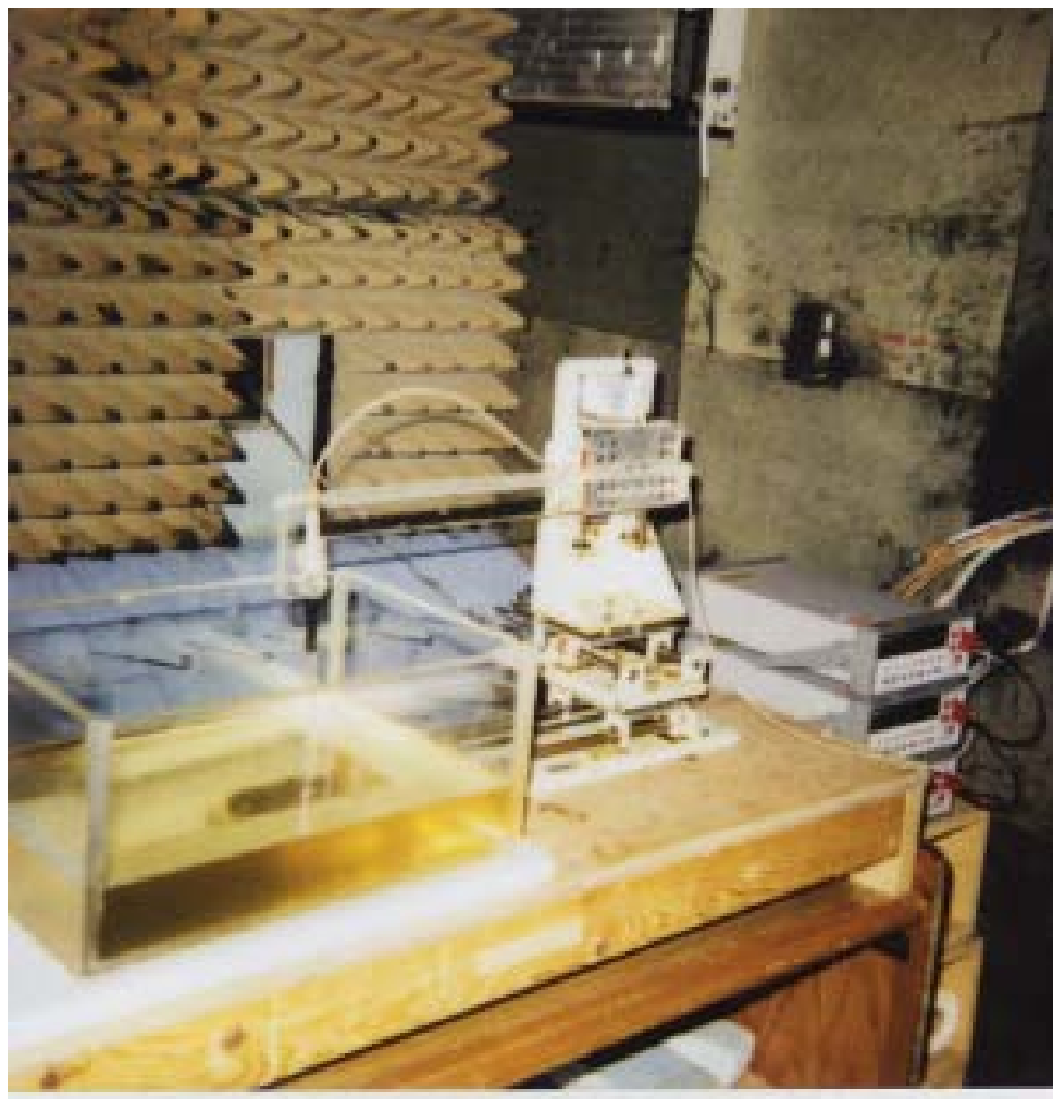
Fig. 4. Photograph of the three-dimensional stepper-motor-controlled SAR measurement system using a planar phantom (see Figs. 3, 6, and 7 for a detailed examination of the placement of Agency Series PP2170 Laptop Computer with Ambit Microsystems 802.11a Wireless Antennas relative to this phantom).
